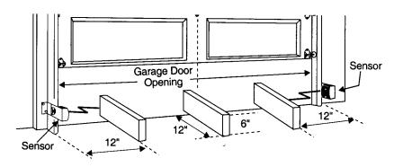
If the door does not respond properly to these tests, the Infrared Safety Sensors must be adjusted (refer to step 22 or 23 depending on type of sensors used). Repeat this test procedure. If the door opener still will not respond properly and fails this test, the door may cause severe injury or death. Have a qualified service person make repairs.
